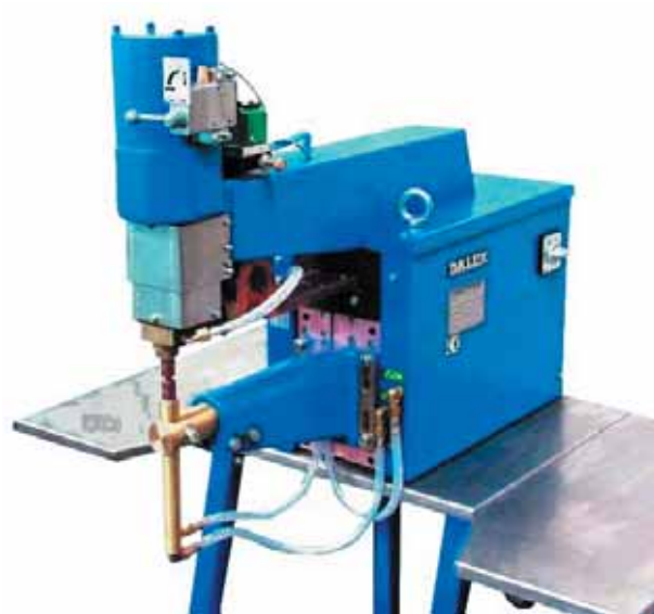
fig. PMS 10-4 T in model A as spot welding machine
